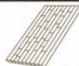
Finger-joint panel with one or two solid lamellas
